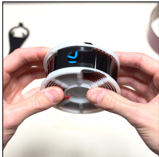
Figure 2.11: Pull the clip toward the start of the spiral until the two tabs hit the plastic
