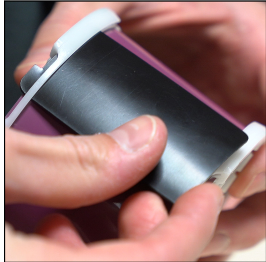
Figure 2.5: Slide the first tab of the clip into the film guide
