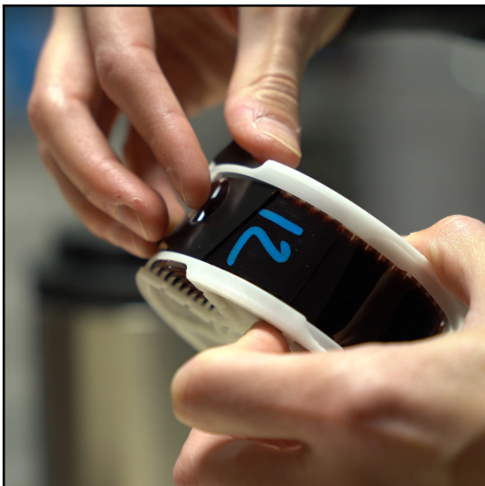
Figure 2.10: Rotate the clip and slide the other side into the other film guide
